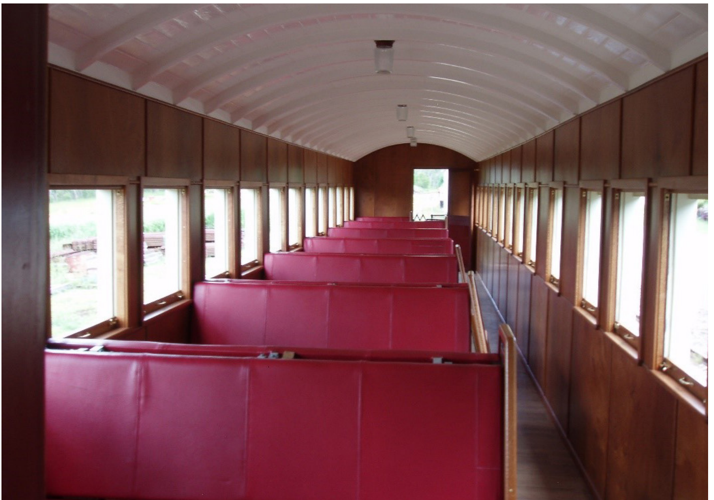
Image: The carriage's interior was lovingly restored using reclaimed silky oak and rare silky oak veneer.
